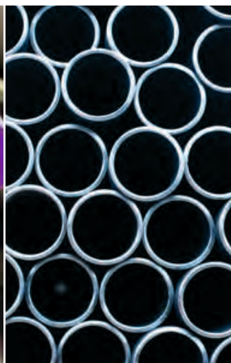
Stainless steel is resistant to corrosion because the steel has been alloyed with, for example, nickel.
